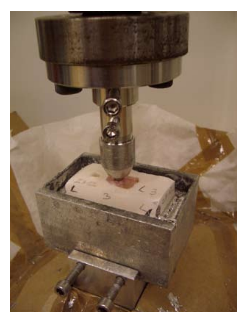
Fig. 6: Setup of mechanical testing. MTS testing machine and a fixed sample
