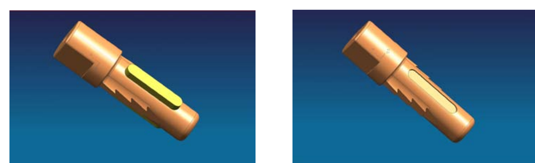
Fig. 3: Left: Test implant with titanium core and two polymer (PLA) stripes (yellow) Right: Control implant type without polymer parts
